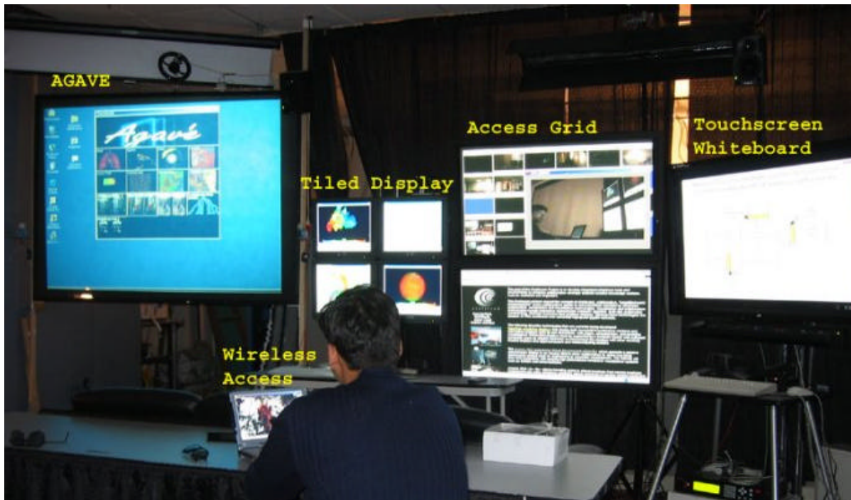
Figure 1. One of two Continuum Amplified Collaboration Environments at the Electronic Visualization Laboratory at the University of Illinois at Chicago. Top left is a collaborative passive stereoscopic display for showing immersive 3D content; next to it is a 2x2 matrix collaborative tiled display; next to it are vertically stacked plasma screens that are used for Access Grid multi-site video conferencing; to the right of this is the plasma touch-screen that is used for shared white-boarding; interaction to these displays via wireless access.
