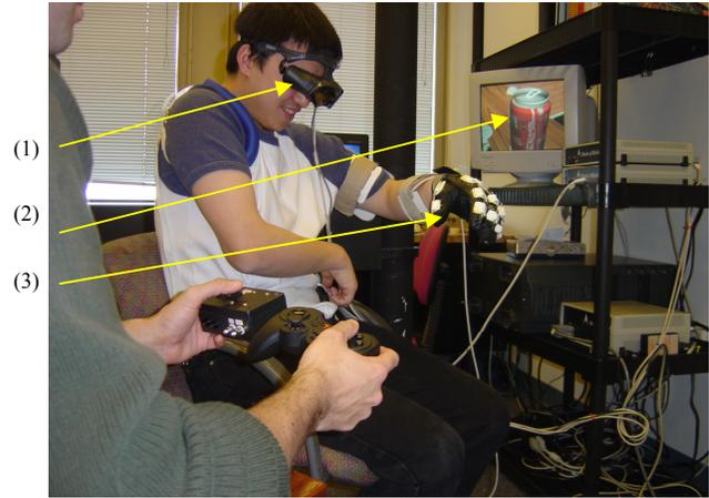
Fig. 1. On-site setup of the training environment using BPO. The therapist is holding both the joystick and control switch (see section D) in his hands. (1): HMD, (2): Fish Tank, (3): BPO.
