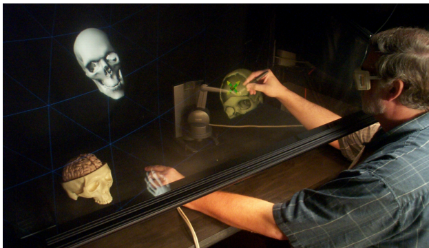
Figure 2. A medical modeler "touches" a cranial defect while sitting at PARIS™. The stylus corresponds to a tool held in the right hand; a virtual hand tracks the position of the left hand. A real model remains visible on the table.
