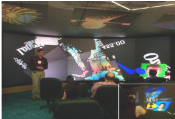
Figure 7. TIDE at SC99: A user running the TIDE Client on a PowerWall, at the ASCI booth. Inset: Another user collaborating from an ImmersaDesk
