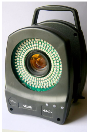
Figure 3-7: Strobe unit (F-series and MX+)
