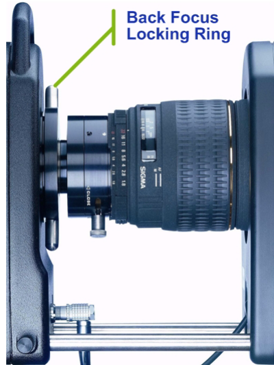
Figure C-6: Camera back focus lock
