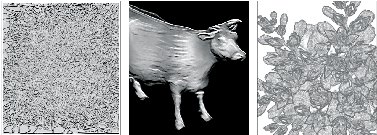
Figure 1. 3D models created with Kizamu (“to carve” in Japanese) and rendered with simple Phong illumination; all texture is purely geometric. On the left – a slab carved with 2000 random chisel strokes (level-12 ADF, 124 MB); in the center – a procedurally sculpted cow; on the right – flowers carved in bas-relief from a slab.
