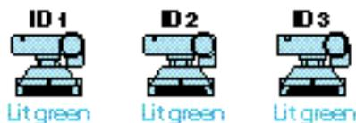
The selection of the VC-C3 with ID number 2 is cancelled and the restriction on the operation of other VC-C3s is removed. The base LEDs on all the VC-C3s turn green and all the VC-C3s can be controlled using the wireless controller.
