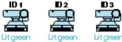
The ID numbers have been set using the ID selector and the base LEDs on all the VC-C3s are lit green.
