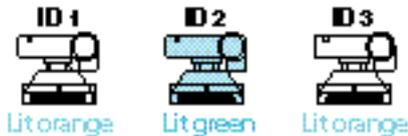
The base LED on the VC-C3 with the ID number equal to 2 turns green to indicate that the VC-C3 is selected. The base LEDs on the VC-C3s with other ID numbers remain lit orange and do not respond to wireless controller commands.
