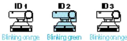
Only the VC-C3 with the ID number 2 can be controlled using the wireless controller. The base LEDs on the VC-C3s with other ID number blink orange (at 0.1-second intervals) and the VC-C3s do not operate.
