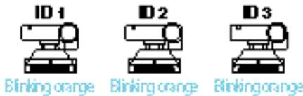
The base LEDs on the VC-C3s blink orange (at 0.5-second intervals).
