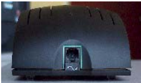
Figure 2-4. Quad BRI Network Interface Module (P-LINK side)
