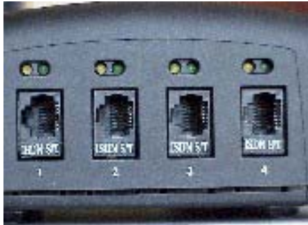
Figure 2-5. Quad BRI Network Interface Module (Network side)
