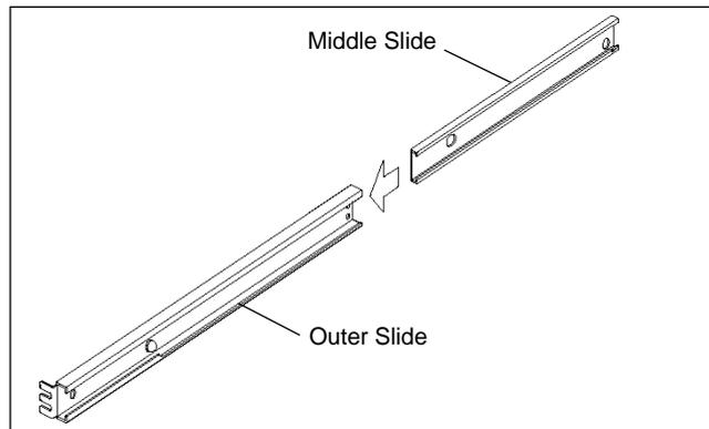
Figure 1. Middle Slide Into Outer Slide
