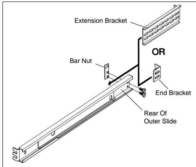
Figure 4. Attach Slide To Bracket
