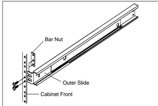
Figure 2. Outer Slide To Cabinet Rack
