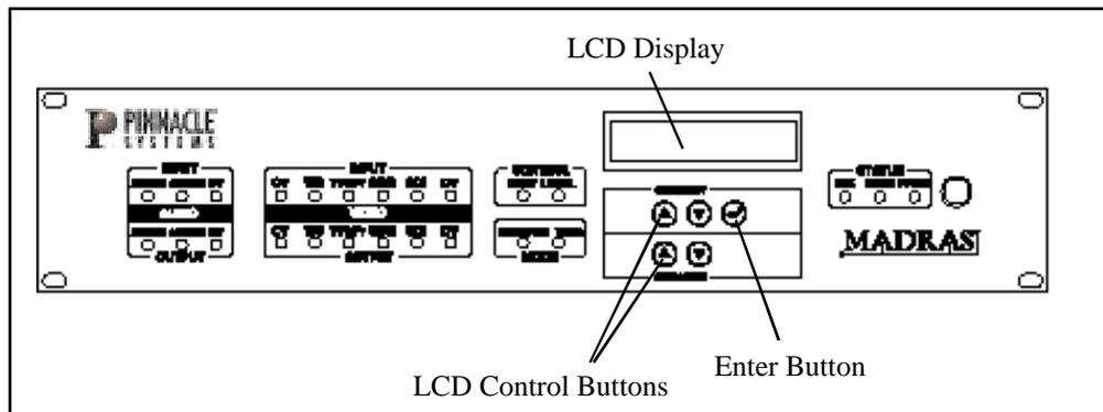
Figure 3-1 LCD Controls
